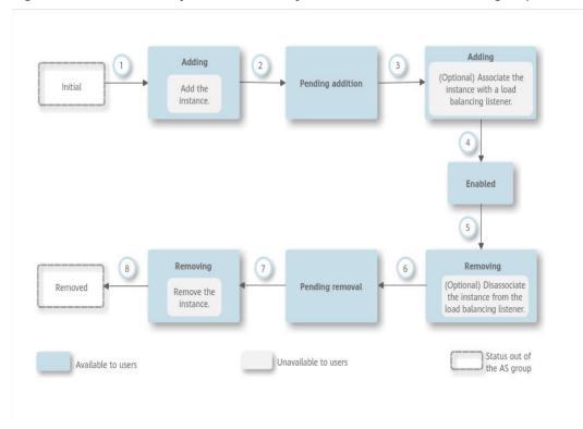
Figure 4-4 Instance lifecycle when a lifecycle hook is added to an AS group
