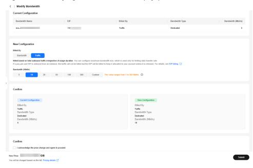
Figure 1-5 Modifying the bandwidth of a pay-per-use EIP
