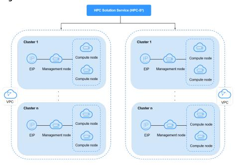
Figure 1-1 HPC-S<sup>2</sup> architecture
