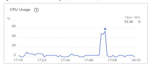
Figure 12-5 broker-2 CPU usage (batch.size = 1 KB)
